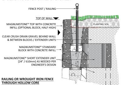
FENCE POST / RAILING TOP OF WALL FENCE POST CORED THROUGH CAP UNIT PLANTING SOIL MAGNUMSTONE® STANDARD **BLOCK WITH CONCRETE INFILL** CLEAR CRUSH DRAIN GRAVEL BEHIND WALL & BETWEEN BLOCKS / EXTENDER UNITS MAGNUMSTONE® STANDARD **BLOCK WITH CONCRETE INFILL** MAGNUMSTONE® SHORT EXTENDER UNIT [24" / 610mm] AS NEEDED PER ENGINEER'S DESIGN **RAILING OR WROUGHT IRON FENCE** THROUGH HOLLOW CORE WITH CAP
